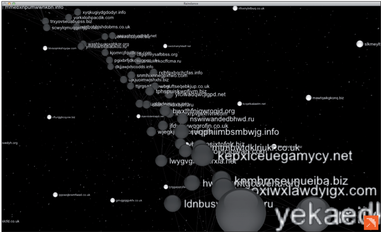
Figure 3: Ripple effect expanding the co-occurrence domains from the set of seed domains with which we started.
